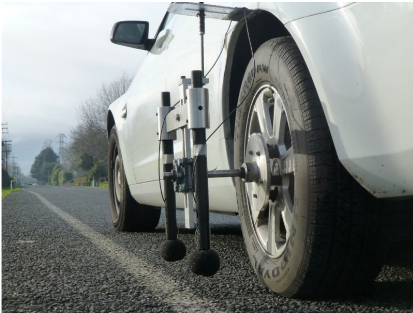
Figure 3.1 Mounting of microphones for close- proximity measurements
