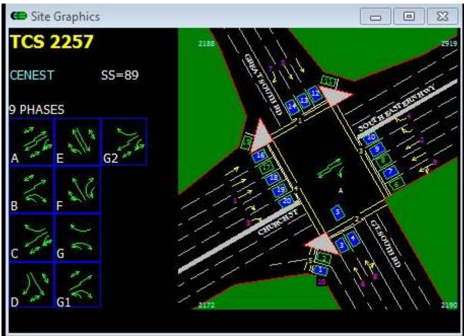
Figure 8.8 Signal phasing for intersection of Church Street and Great South Road Auckland (Auckland Transport)
