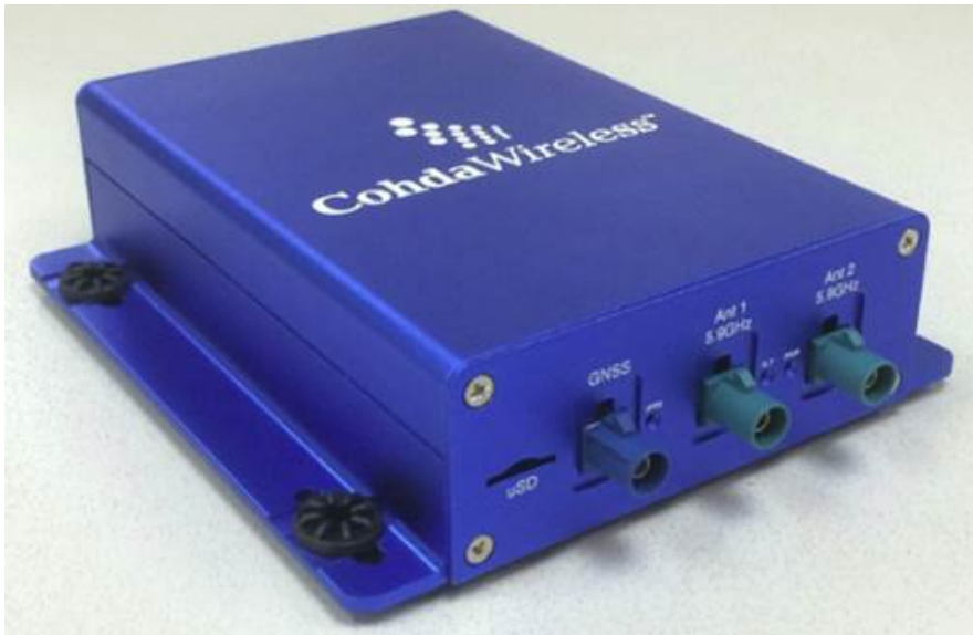
Figure 8.19 Cohda dedicated short- range communications device
