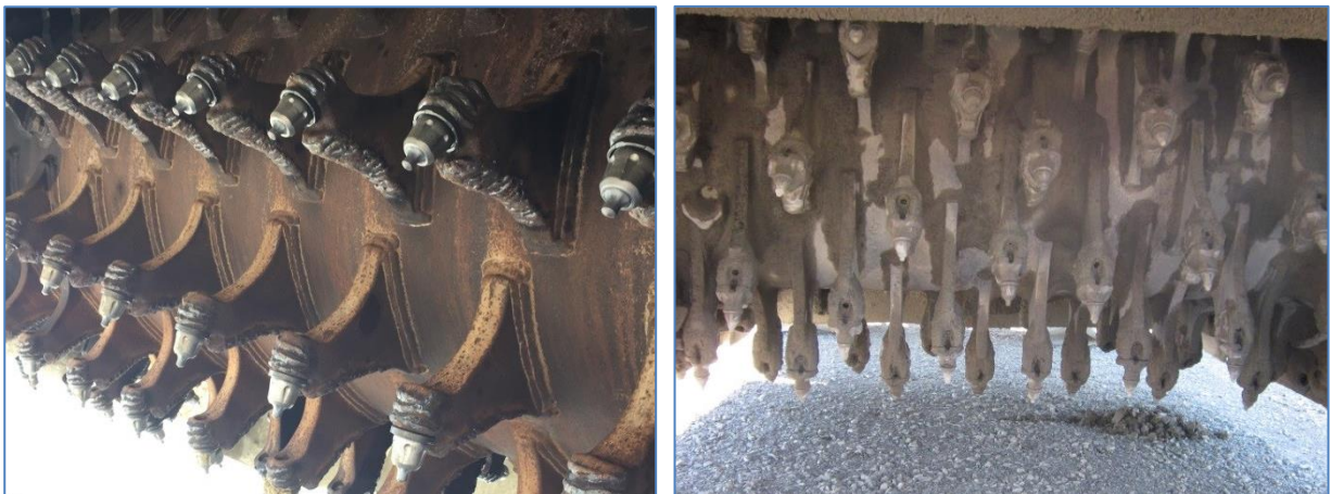
Figure 6.2 Different teeth and drum arrangements on modern pavement stabilisers
