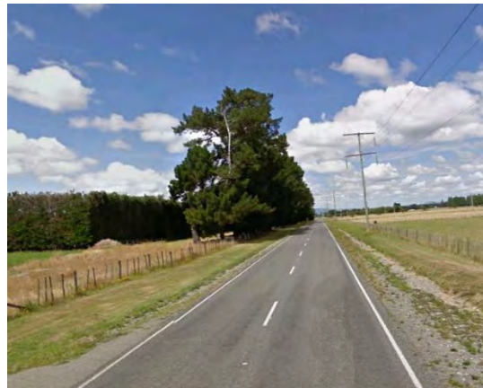
Targeted EMP: Straight road after intervention without EMPs, but with RRPMS, edgelines and centrelines
