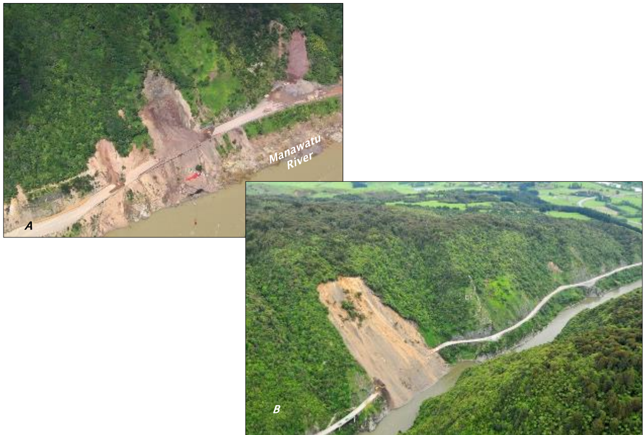
Figure A.29 Large landslides triggered by rainstorms closed SH3 in the Manawatu Gorge for 3 months in 2004 (A), and at another site for 13 months in 2011 (B). A large earthquake could trigger similar landslides at a number of sites within the gorge where the steep marginally stable slopes have been cut back for road widening.
