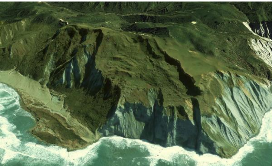
Figure A.27 Google Earth image (2004) of a very large ( \sim 30\text{Mm}^3 ) partly-developed rotational (coherent) landslide in Tertiary mudstone on the \sim 150\text{--}250\text{m} high cliffs at Cape Turnagain on the Wairarapa coast. This landslide may have occurred in 1855 and was reactivated during the 1904 Cape Turnagain earthquake.
