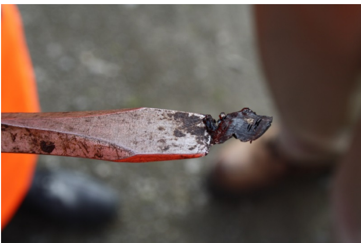
Figure 3.3 Binder is plastic rather than brittle
