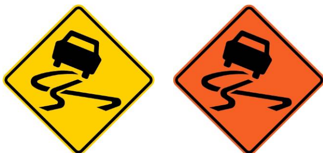
Figure 2.1 New Zealand permanent (code WR3) and temporary (code TR2) slippery road surface signs
