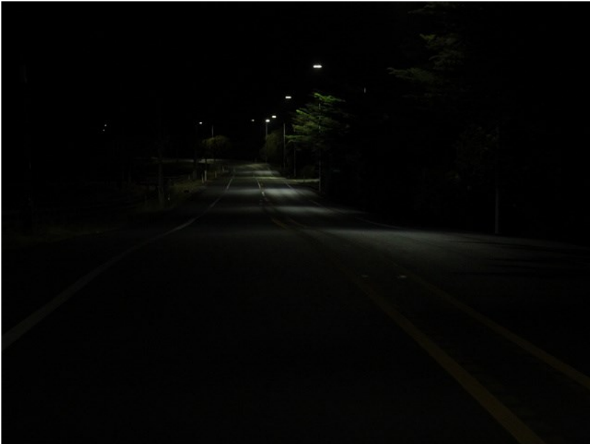
Figure D.6 A lighting scheme with a very high average luminance near the top end of the sample's distribution for both average luminance and uniformity [ \bar{L} = 1.6 , U_o = 0.65 , UI = 0.72 ]
