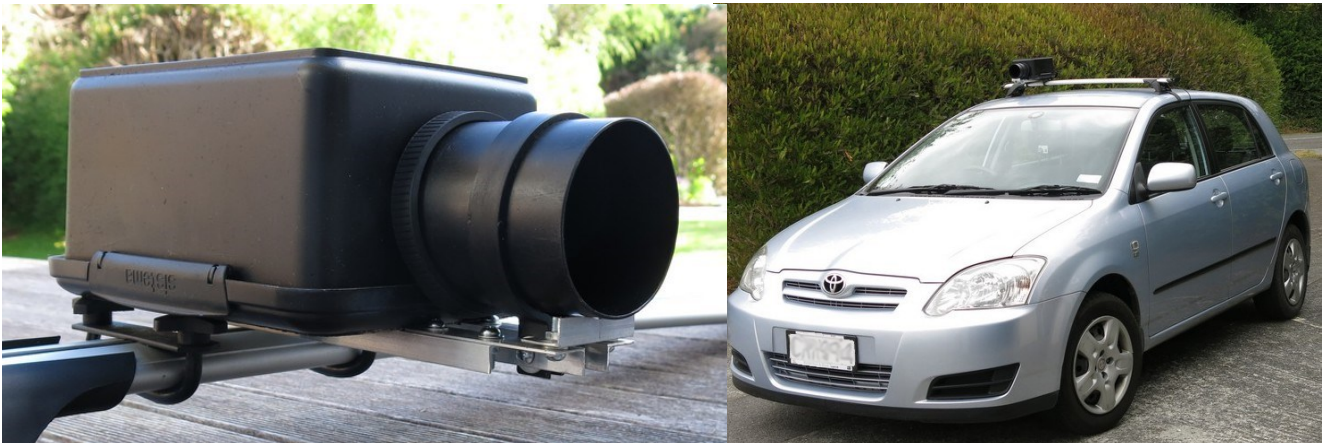
Figure 8.3 (a) Camera inside its weatherproof container and attached to a single car roof bar, (b) Survey vehicle with camera and bar attached
