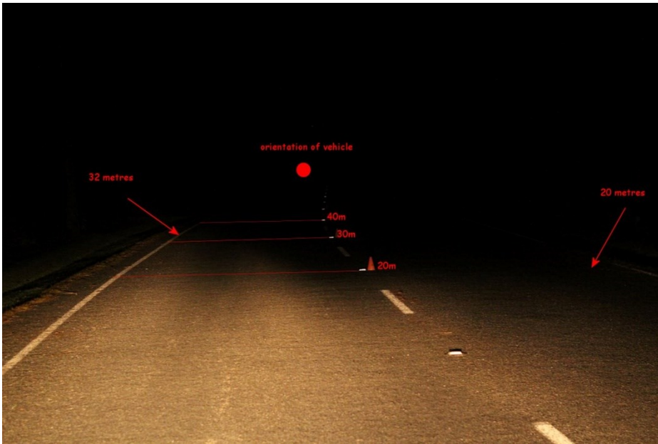
Figure 8.1 Headlight test on a flat level road which showed the survey car's headlights to have no measureable influence on road luminance beyond the point 40m forward of the driver
