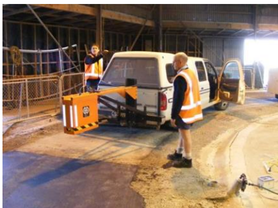
Figure 2.16 Air launched ground penetrating radar
