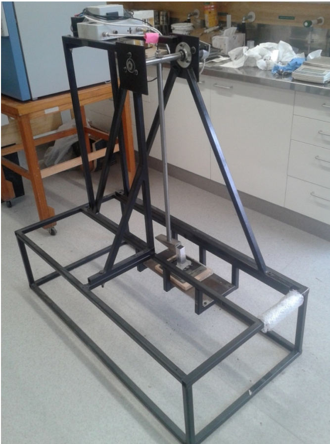
Figure 4.1 Opus Research pendulum tester with chipseal sample in place
