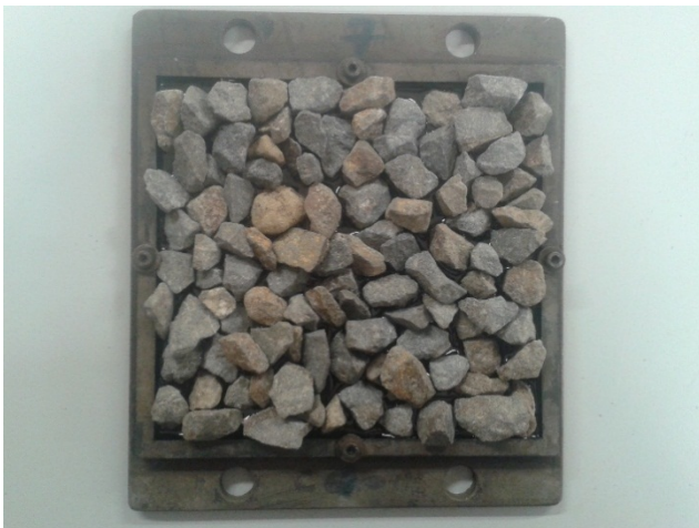
Figure 4.10 1.93Lm 2 bitumen base binder A, Grade 3 chip
