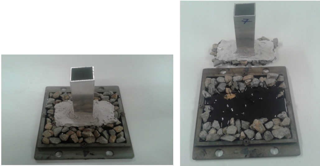
Figure 4.3 Chipseal plate with tower attached and after knock-off
