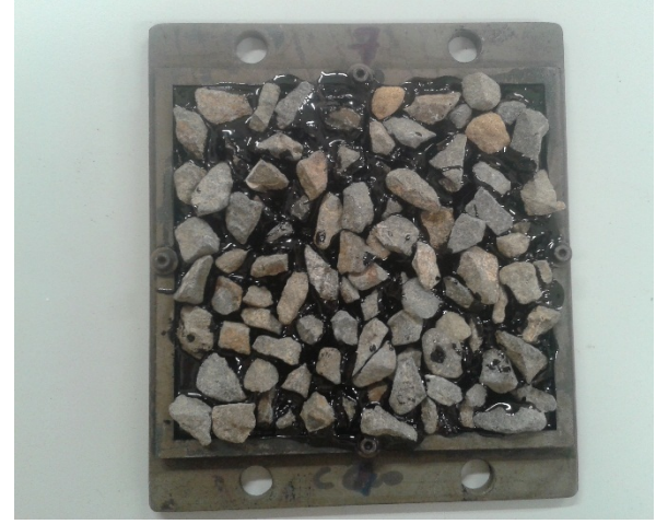
Figure 4.9 3.0Lm 2 emulsion A, Grade 3 chip
