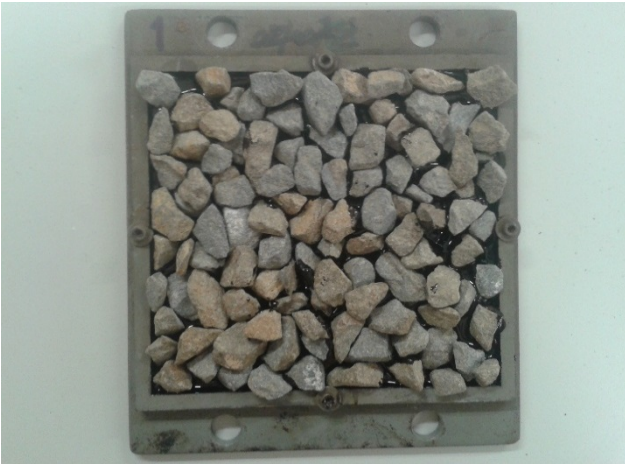
Figure 4.8 1.93Lm 2 emulsion A, Grade 3 chip
