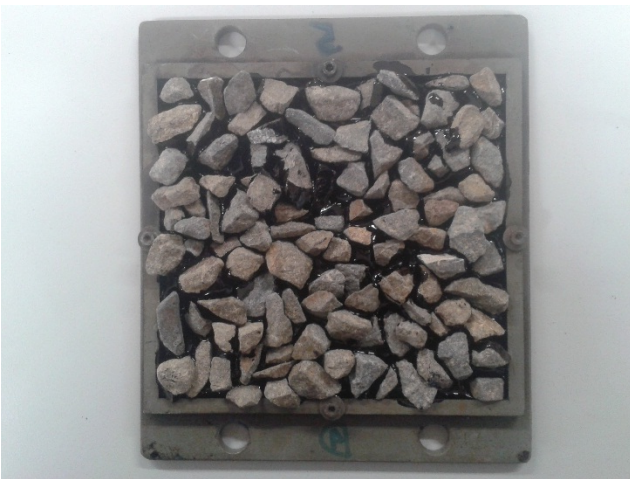
Figure 4.10 1.93Lm 2 bitumen base binder A, Grade 3 chip
