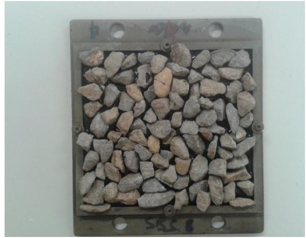
Figure 4.9 3.0Lm 2 emulsion A, Grade 3 chip
