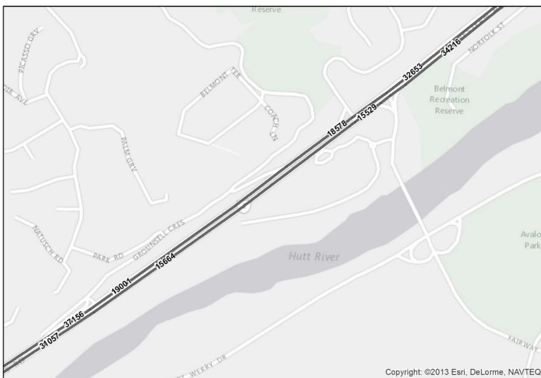
Figure 8.4 Example of incorrect AADT values on CAS centreline (SH2 Wellington)
