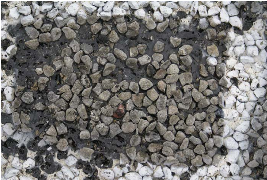
Figure 8.9 Test patch the day after construction showing chip loss through cohesive failure of the binder
