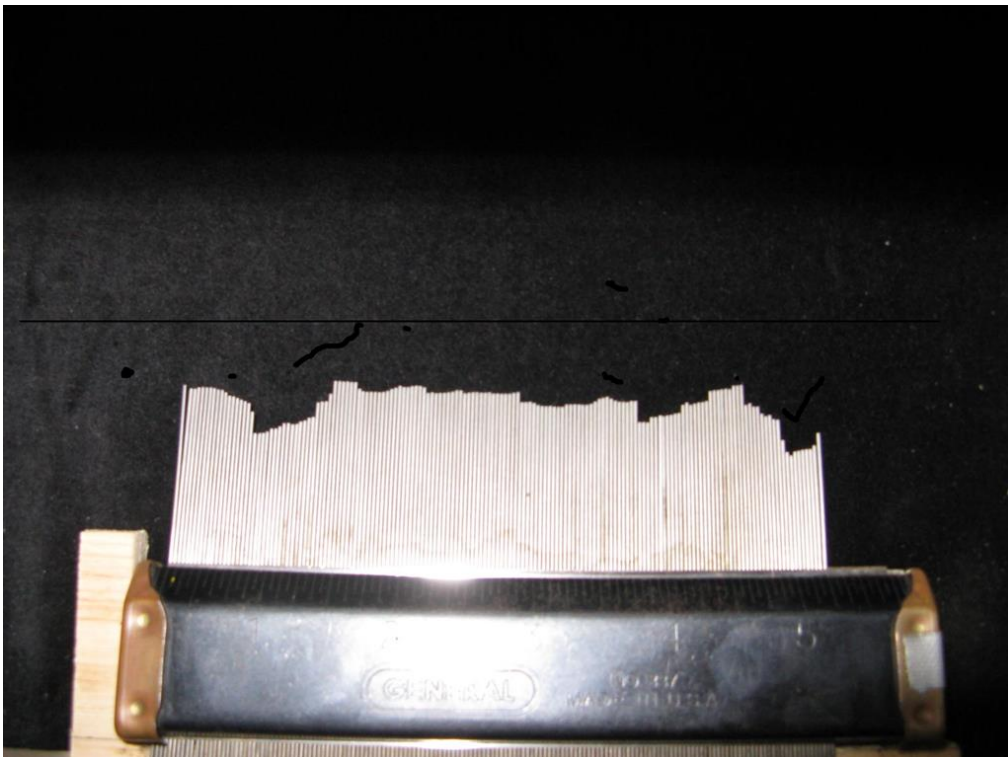
Figure 2.2 Pin profiler device used to measure texture depth
