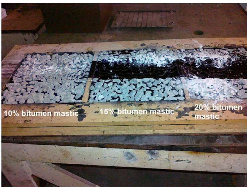
Figure 4.1 Effect of differing proportions of bitumen in the mastic composition after about six hours tracking. The white material apparent on the chips is talcum powder used to minimise bitumen adhering to the tyre
