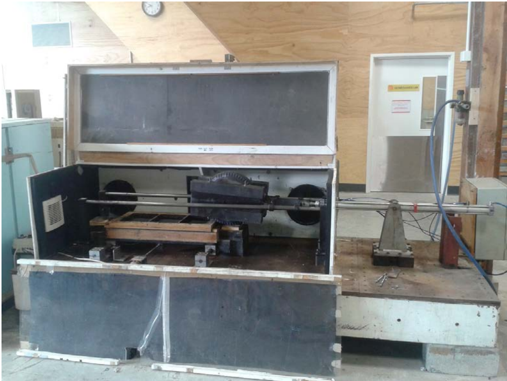
Figure 2.2 Pin profiler device used to measure texture depth
