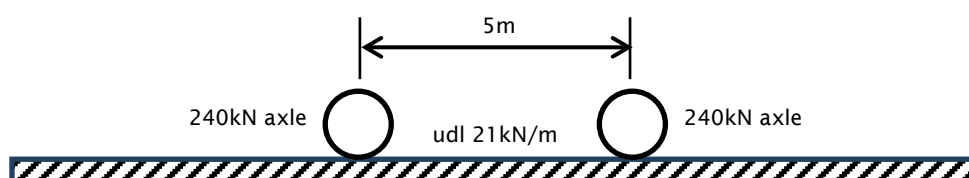
Figure D.13 Bridge manual HN-72 loading factored to represent the design actions from TT73 vehicles (2.0_HN)
