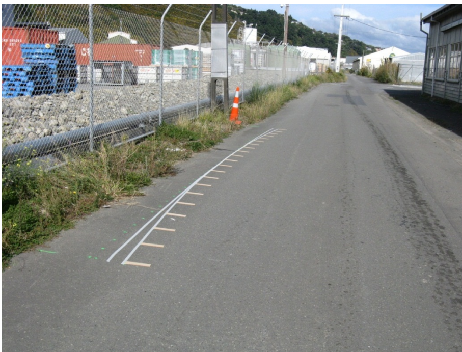
Figure 5.4 Example test-run layout showing a 10-metre length at 50m radius with ribs 9mm high at 500mm spacing
