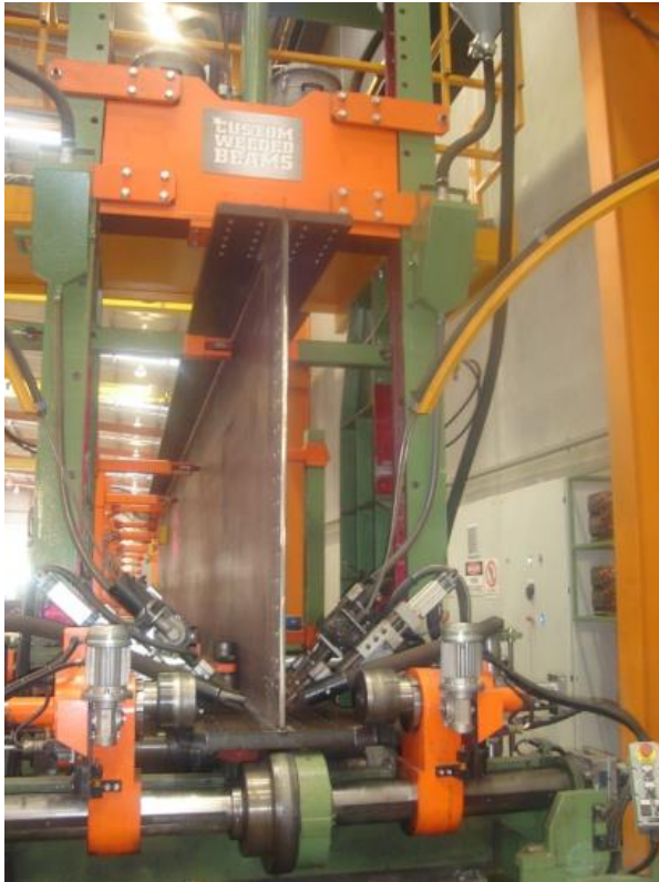
Figure 4.1 Example of a semi-automatic girder welding machine (image courtesy of D&H)
