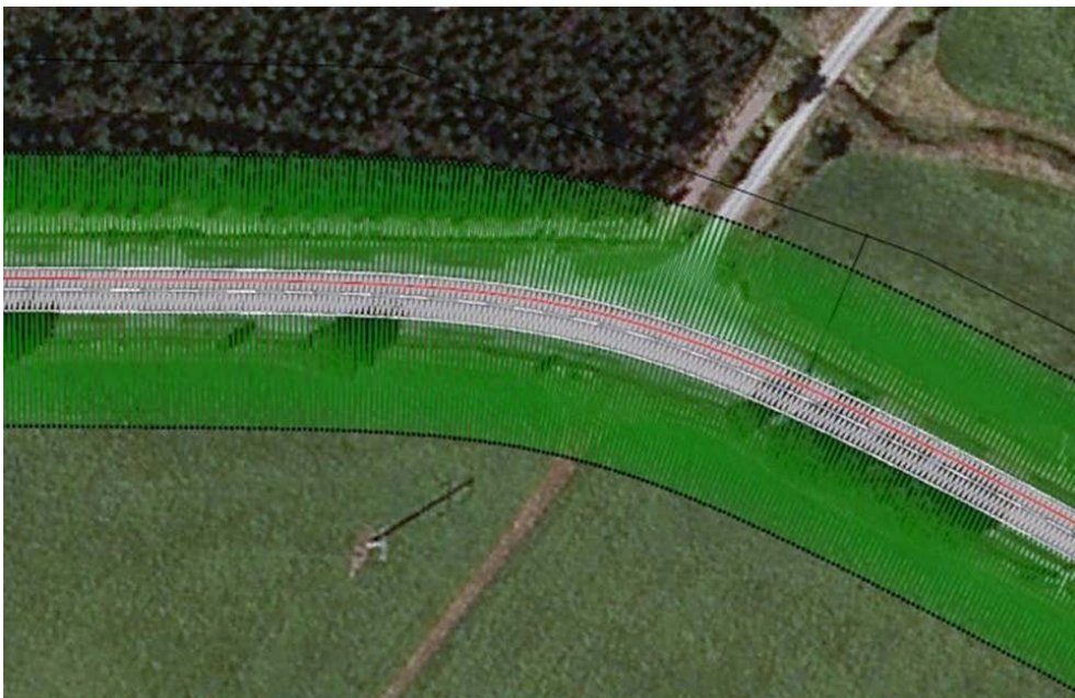
Figure 5.2 Plan view of 3D road corner model (red line - mid-lane follow path)
