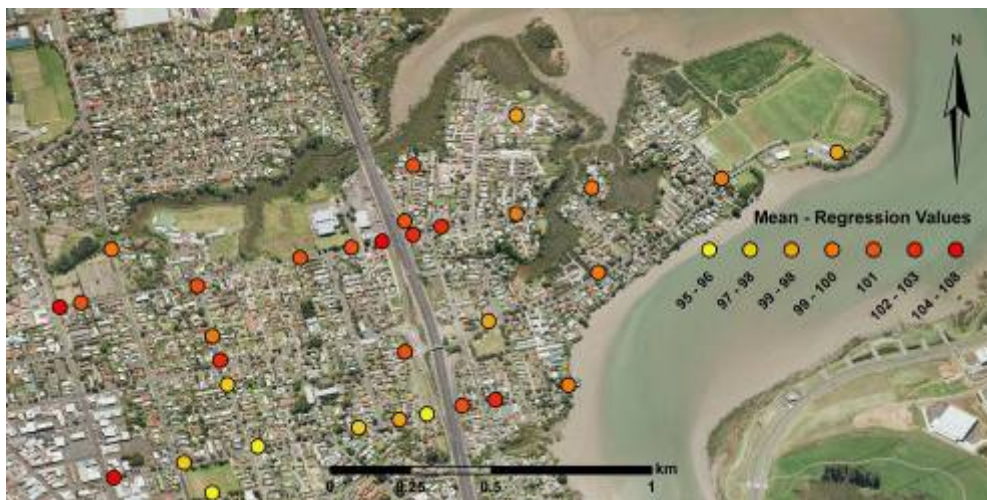
Figure A10.3 Difference between actual mean measured and LUR predicted NO 2 values (Obs-Exp) at monitoring sites for Otahuhu
