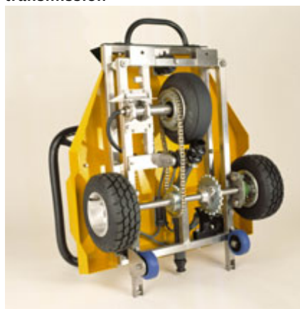
(b) GripTester measuring wheel & chain transmission
