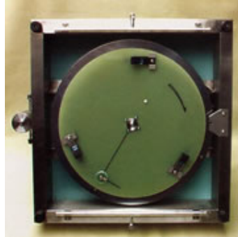
(b) DF Tester spinning disk and rubber sliders
