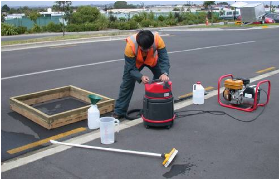
Figure 3.14 Pavement surface detritus sample collection method
