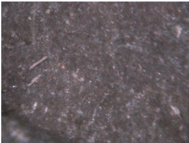
Figure 8.19 Otaika greywacke – after polishing with various contaminants (approx. field of view 3.5 x 2mm)
