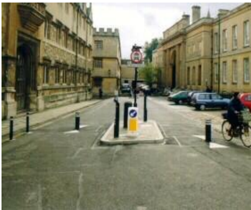
Bus gate enforcement using raised bollards Source: AECOM 2010
