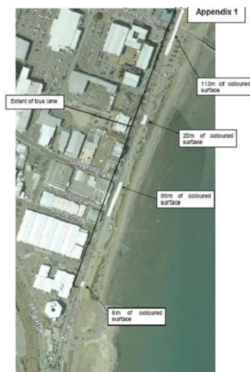
Figure A5.11 Petone Esplanade special vehicle lane (Source: MWH 2005)
