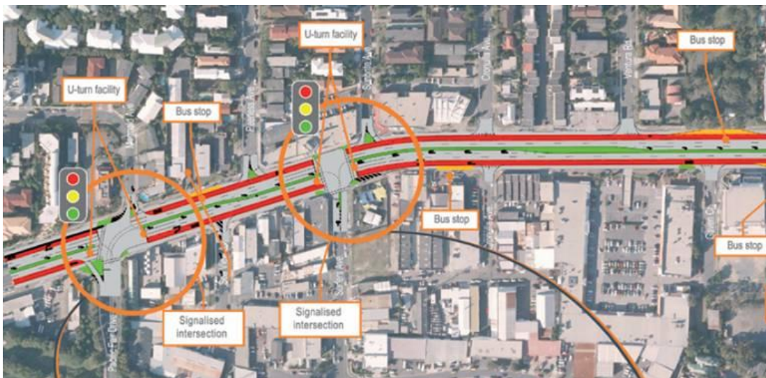
Figure A5.19 Layout of additional bus lanes and upgrade to traffic signals
