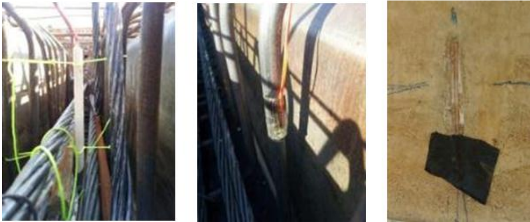
Figure 5.5 Strain gauges installed during construction
