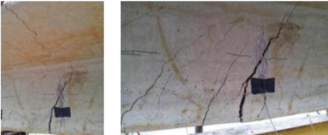
Figure 5.14 Web cracking behaviour of unit 40-10-A
