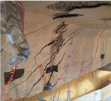
(b) Crack pattern at failure
