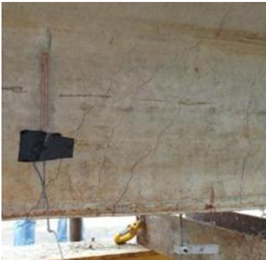
Figure 5.9 Web cracking behaviour of unit 40-8-A
