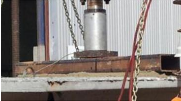
(a) Load jack with load cell attached
