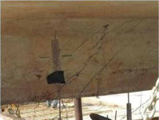
Figure 5.26 Web cracking behaviour of unit 80-8-A
