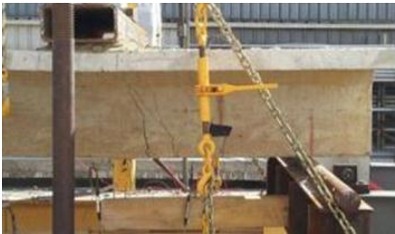
(a) Dominant crack during loading
