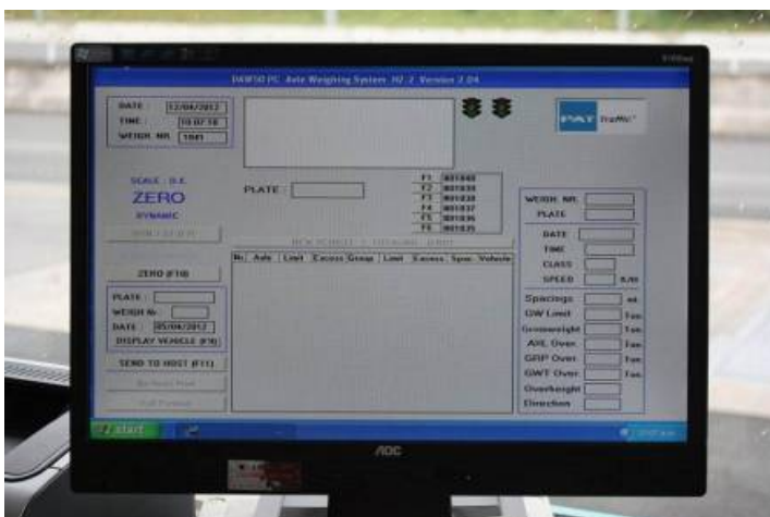
Figure 7.4 Image of current New Zealand Police CVIU slow-speed WIM operator screen (Plimmerton Weigh Station)
