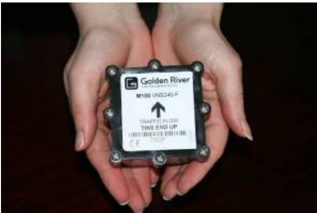
Figure 7.3 Image of wireless magnetometer (courtesy of Clearview Traffic)
