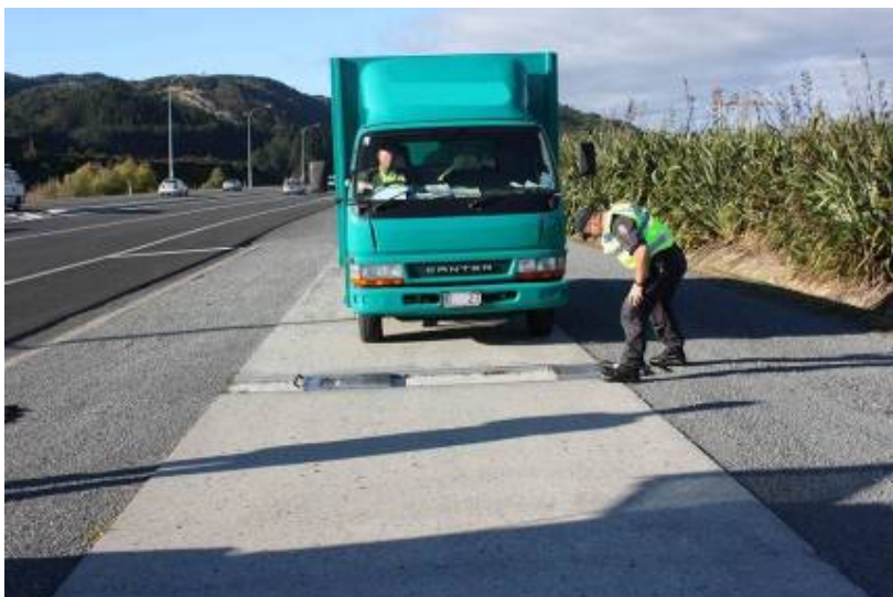
Figure 2.6 Weigh pit HCV inspection, using portable static scales
