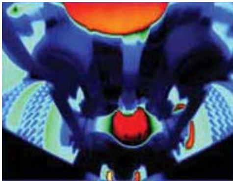
Figure 7.7 Under-vehicle FLIR image showing uneven brake temperature (courtesy of Bill Legg, WSDoT)
