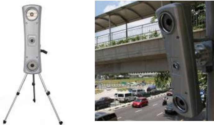
Figure 7.1 3D camera used in Project Asset in portable tripod mounted and fixed format (courtesy of KRIA 7 )
