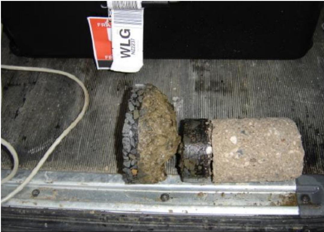
Figure E.59 A core from the over-layered section at SH38 0/1.935
