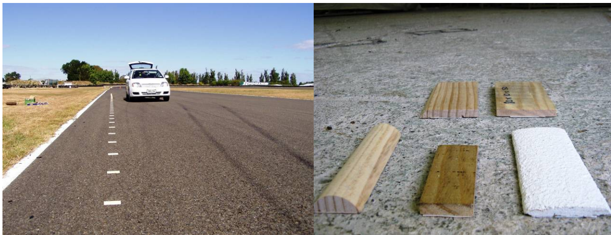
Figure 2.1 The test car next to a line of test blocks on the Manfeild race track, and a selection of five test blocks, including four wooden test blocks and one thermoplastic test block
