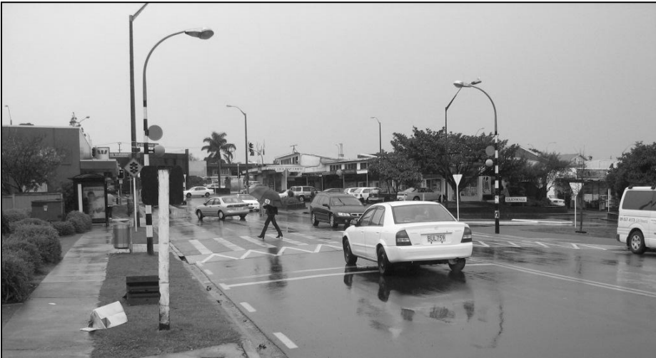
Figure 7.2 A typical speed platform with a zebra crossing installed in Glen Eden town centre, Waitakere
