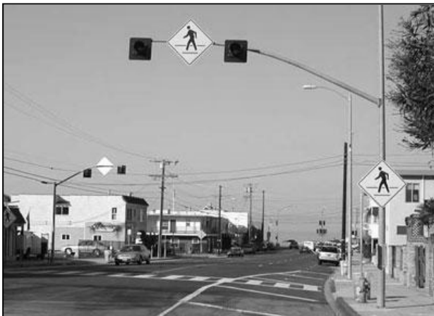
Figure 5.8 RRFB signage used in the US (Malek 2001)
