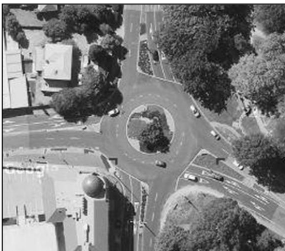
Figure 3.11 Example of a roundabout built with minimal regard for speed control: Riccarton Road and Deans Avenue in Christchurch (photos courtesy of Google Maps)
