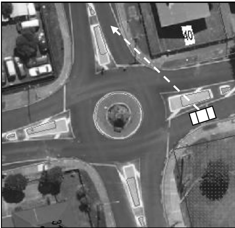
Figure D1 Birds-eye view of the Church Street–Avenue Road roundabout in Otahuhu, Auckland, showing how sightlines are restricted from one approach
