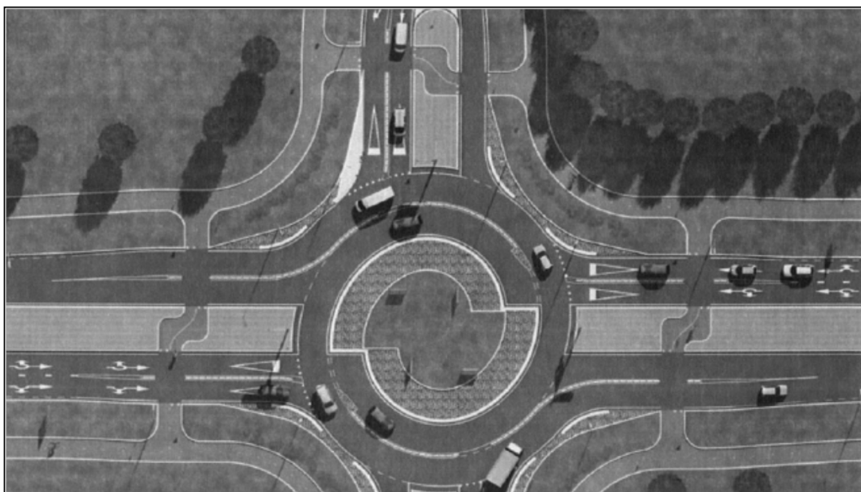
Figure 11 Standard layout of a turbo roundabout
