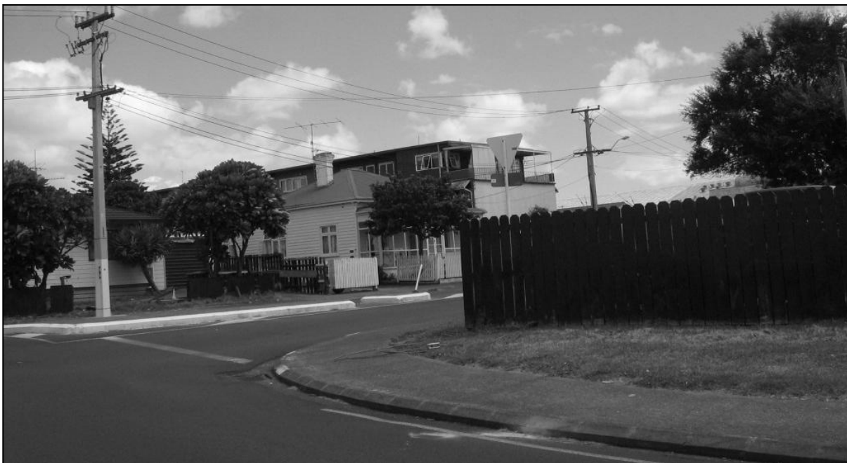
Figure 4.13 View taken on approach C at a point 10m from the roundabout limit line, showing the corner boundary fence which severely restricts visibility of opposing vehicles coming from approach B to the right
