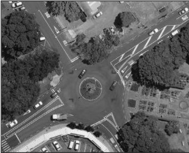
Figure 3.10 Example of a roundabout built with minimal regard for speed control: Pages Road, New Brighton Road, Owles Terrace and Seaview Road in Christchurch (photos courtesy of Google Maps)
