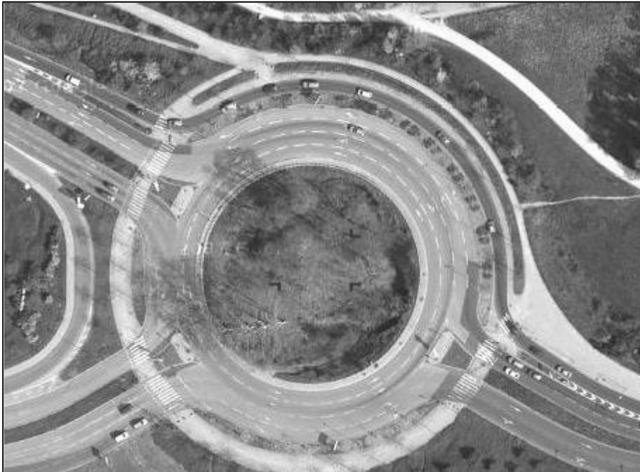
Figure 2.8 A signalised roundabout in Villeurbanne, France (aerial photo courtesy of Google maps)
