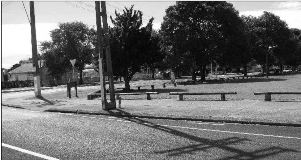
Figure 4.11 View taken on approach A at a point 25m from the roundabout limit line, showing the almost unimpeded visibility of opposing vehicles coming from approach D to the right
