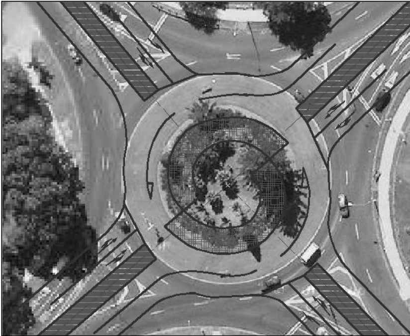
Figure 8.51 A turbo-roundabout layout as per Dutch specifications atop the Robertson Road-Bader Drive roundabout in Mangere, Auckland
