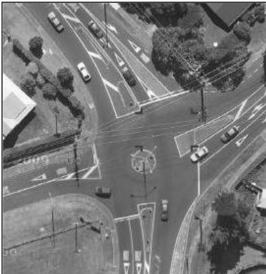
Figure 3.8 Example of a roundabout built with minimal regard for speed control: Glenfield Road and Coronation Road in the North Shore, Auckland (photo courtesy of Google Maps)
