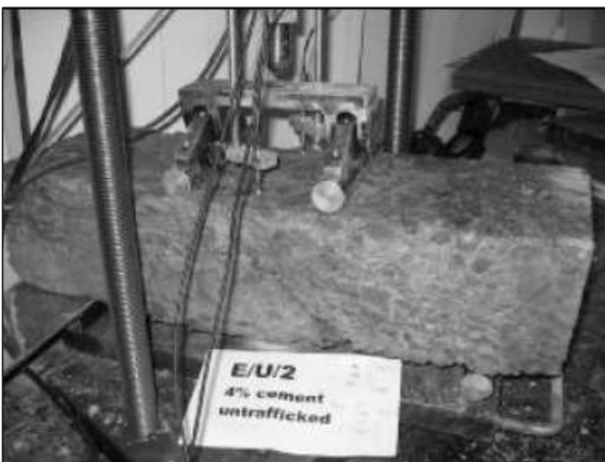
Figure B31 Beam EU2 (saw-cut CAPTIF + 4% cement) at breakage
