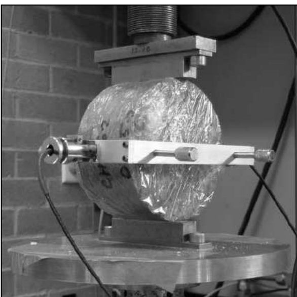
Figure 2.2 IDT equipment: detail (photo courtesy of Austroads (2008))
