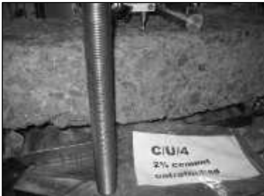
Figure B20 Beam CU4 (saw-cut CAPTIF + 2% cement) at breakage during the modulus test
