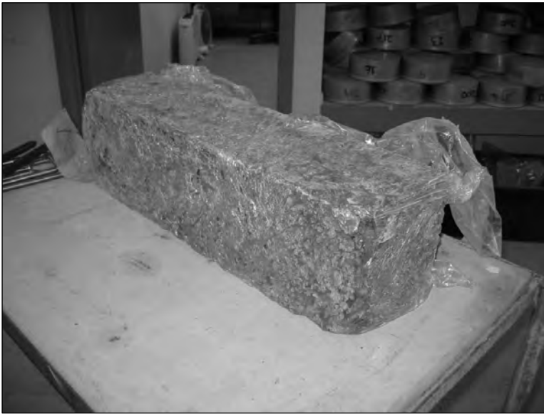
Figure 5.3 Compacted and cured beam ready for testing
