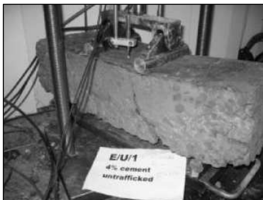
B26 Beam EU2 (saw-cut CAPTIF + 4% cement) at breakage during the modulus test
