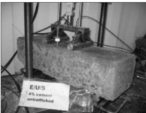
Figure B34 Beam EU5 after two million cycles
