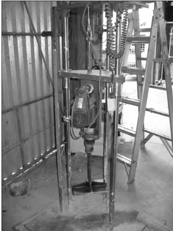
Figure 5.2 Compaction frame with vibrating hammer and foot for beam manufacture
