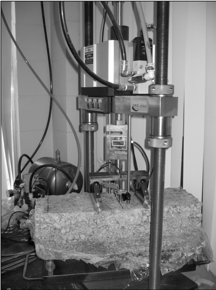
Figure 5.7 Measuring deflection during the flexural beam test using LVDTs
