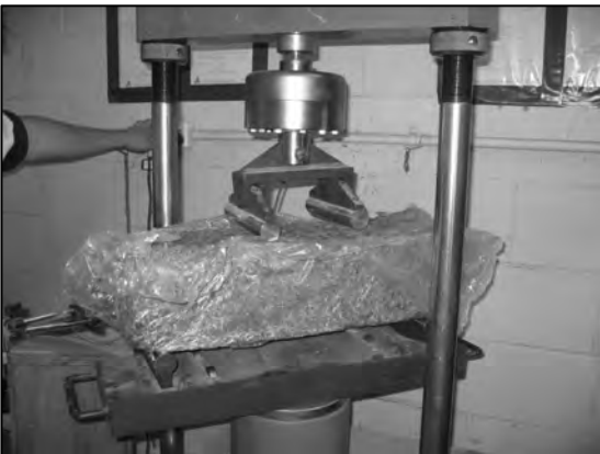
Figure 5.4 Initial beam breakage test, with the beam before breaking
