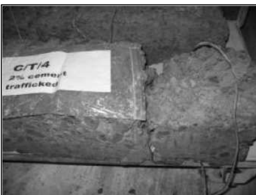
Figure B23 Beam CT4 (saw-cut CAPTIF + 2% cement) at breakage during handling
