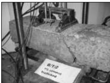
Figure B16 Beam BT2 (saw-cut CAPTIF + 1%) at breakage during the modulus test
