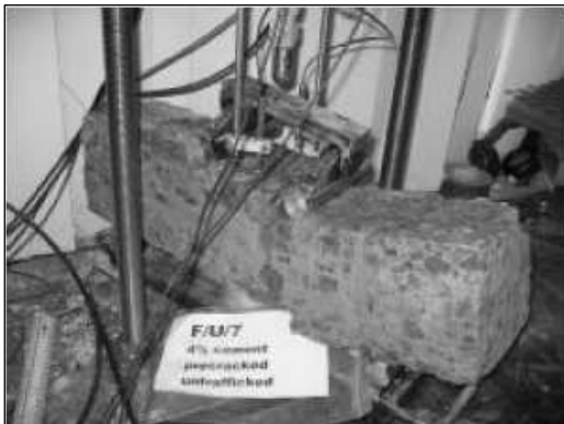
Figure B39 Beam FU7 (saw-cut CAPTIF + 4% concrete, pre-cracked) at breakage during flexural beam modulus testing
