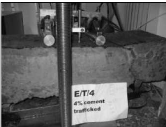
Figure B35 Beam ET4 (saw-cut CAPTIF + 4% cement) at breakage during the flexural beam modulus test
