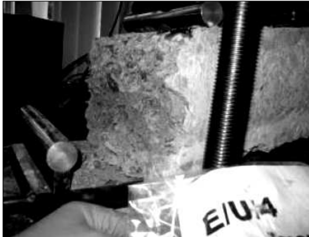
Figure B32 Beam EU4 (saw-cut CAPTIF + 4% cement) at breakage
