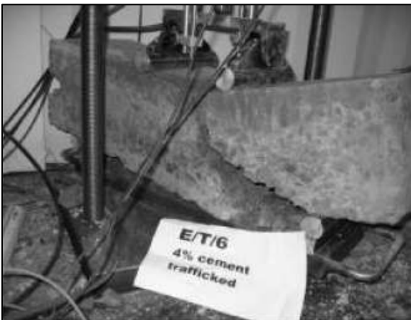
Figure B36 Beam ET6 (saw-cut CAPTIF + 4% cement) at breakage during the flexural beam modulus test
