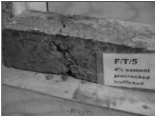
Figure B43 Beam FT7 (saw-cut CAPTIF + 4% cement, pre-cracked) at breakage during flexural beam modulus testing
