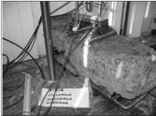
Figure B42 Beam FT5 (saw-cut CAPTIF + 4% cement, pre-cracked) at breakage during flexural beam modulus testing
