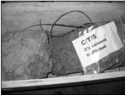
Figure B24 Beam CT5 (saw-cut CAPTIF + 2% cement) at breakage during handling
