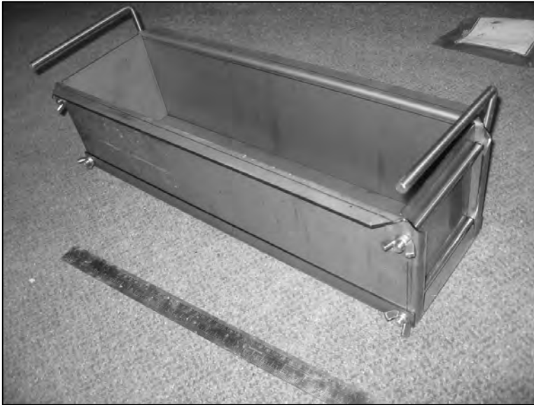
Figure 5.1 Beam mould used for the 530mm × 150mm × 150mm beams
