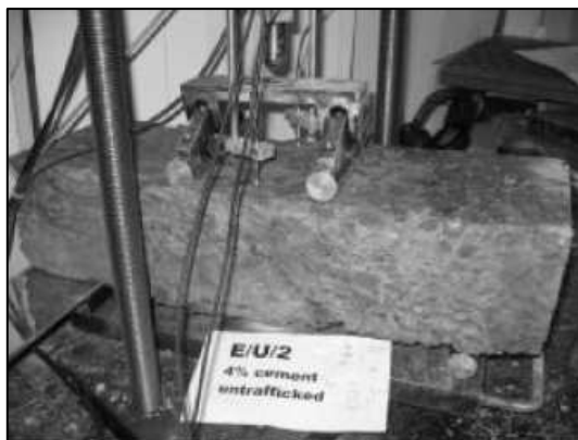
B26 Beam EU2 (saw-cut CAPTIF + 4% cement) at breakage during the modulus test
