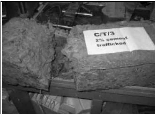
Figure B22 Beam CT3 (saw-cut CAPTIF + 2% cement) at breakage during handling
