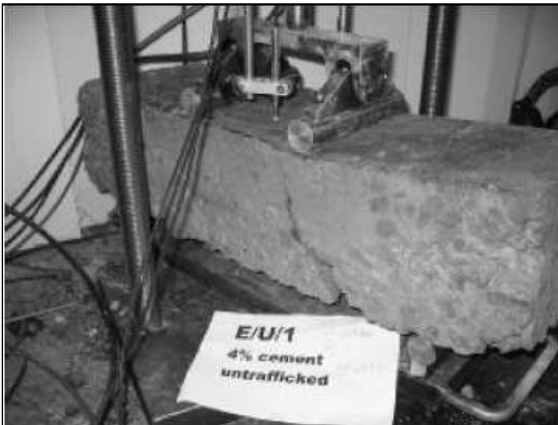
Figure B30 Beam EU1 (saw-cut CAPTIF + 4% cement) at breakage
