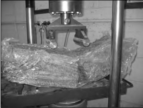
Figure 5.5 Initial beam breakage test, with the beam at breaking point
