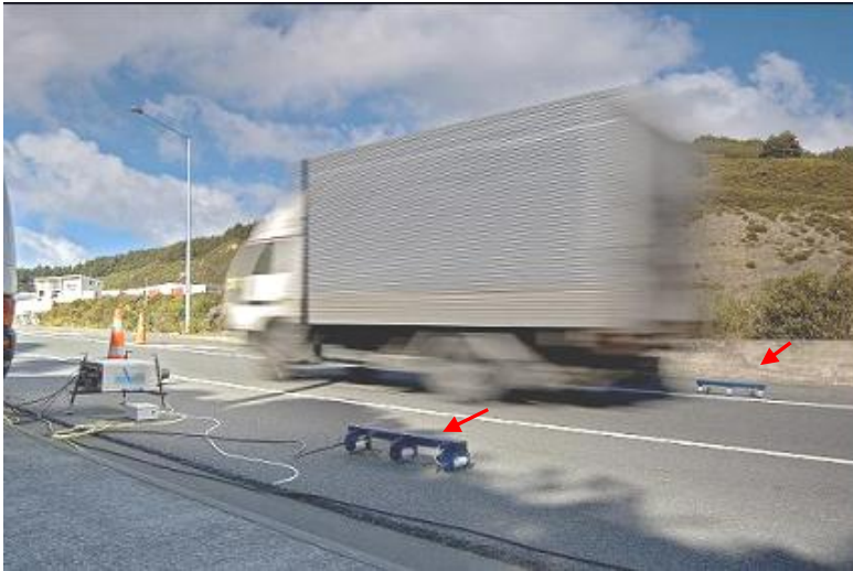
Figure 2.4 The speed and acceleration bars (see arrows) in the RSD system
