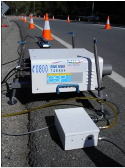
Figure 2.2 Source detector module and calibration unit of the RSD 4000EN
