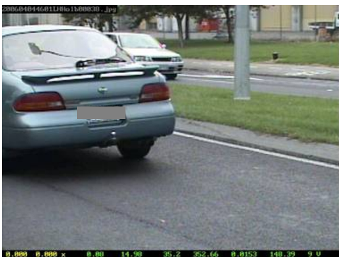
Figure 2.7 Example of a licence plate image recorded by the RSD system
