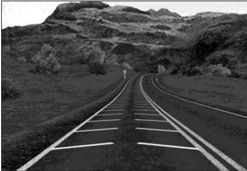
Figure 2.2 Transverse road marking used in a simulator trial (Charlton 2003)
