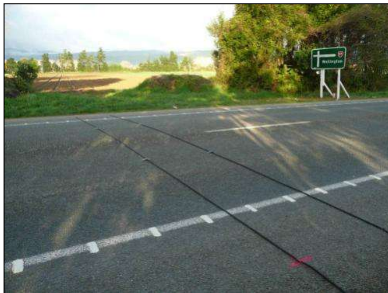
Figure 3.7 Example of typical speed tube set-up, including spray-painted nail holes
