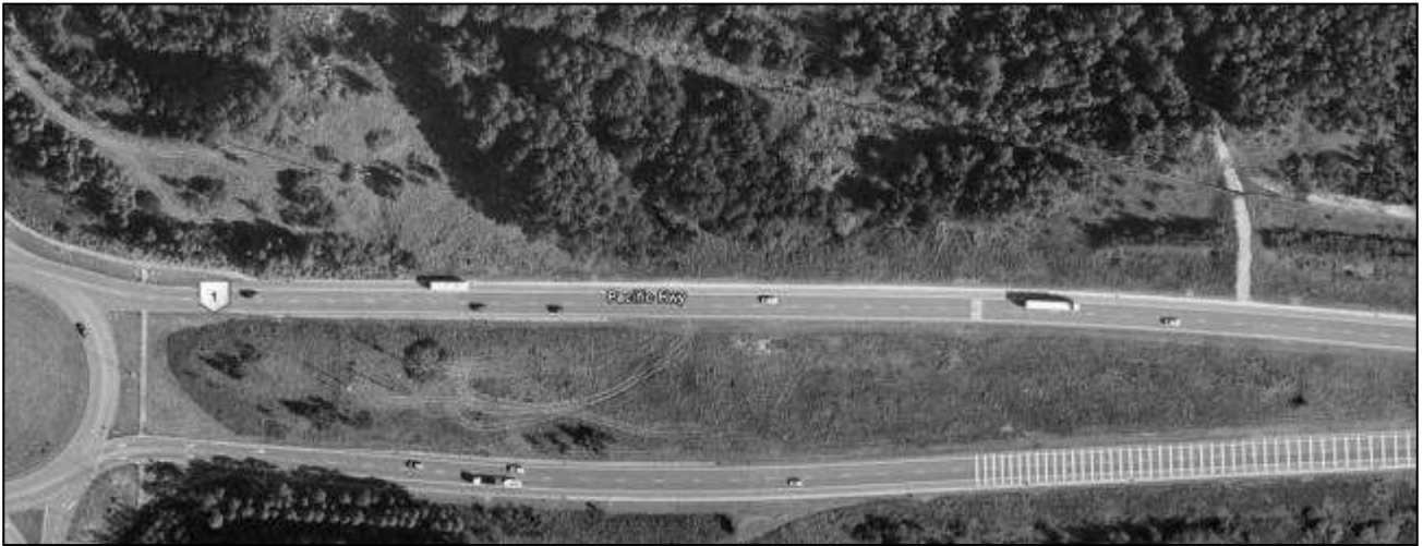
Figure 2.7 Transverse road markings used as a speed deterrent from a 100km/h to 70km/h speed zone on the Pacific Highway in New South Wales, Australia (photo courtesy of Google Earth Pro License)
