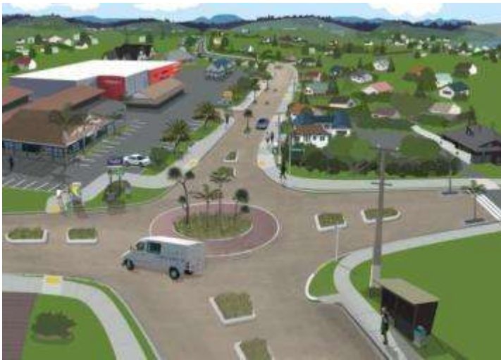
Figure 4.14 In addition to variable active speed-warning signs, consistently designed roads near and outside schools could be designed using SER principles, such as extra-wide footpaths, narrow traffic lanes, minimal road marking, gateway treatments, and planting on the road reserve, to create inherently low-speed environments that might be applied to school zones. Consistent use of crossing design, textured surfacing and roadmarking could be used to create a consistent arterial ‘school zone’ format around schools (Photos/pictures: Dale Projects, Hamish Mackie, Jennifer Esterman)
