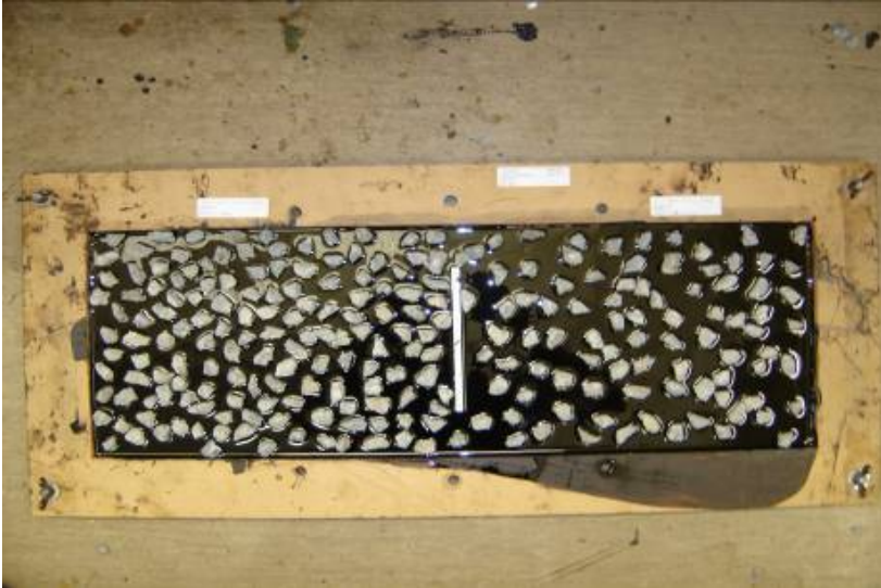
Figure 4.4 Two application rates of grade 3 chip and open bitumen windows
