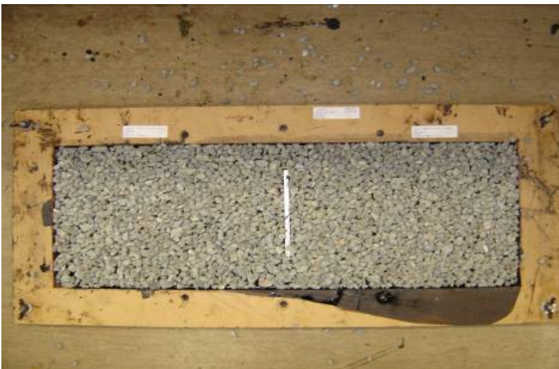
Figure 4.5 Second application using a grade 5 sealing chip
