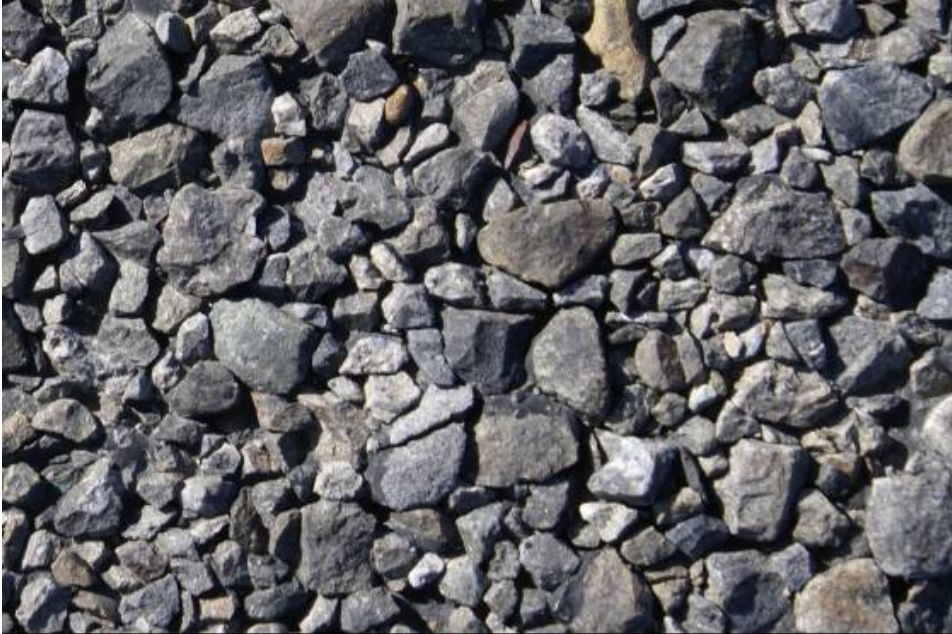
Figure 4.6 Close up of the interlocking of the two grades of chip after 200 passes of the SCR
