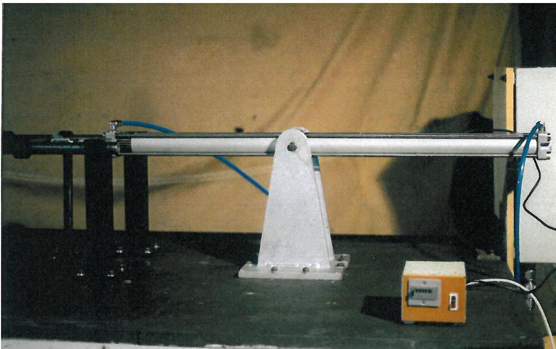
Figure 4.2 Close up of the pneumatic cylinder for longitudinal movement
