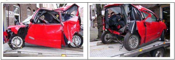
Figure 3.10 Aixam hit from behind by an Audi A6 travelling at 100km/h (www.rijnders-minicars.nl)
