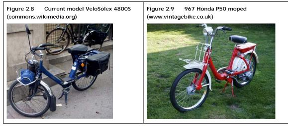
Some mopeds, such as the Honda shown in figure 2.9, were effectively hybrids. This Honda has a power output of 900W, a top speed of 40km/h, and a claimed fuel consumption of 90km/l. Note that in both cases, the claimed fuel consumption and speed are for engine-only operation.
