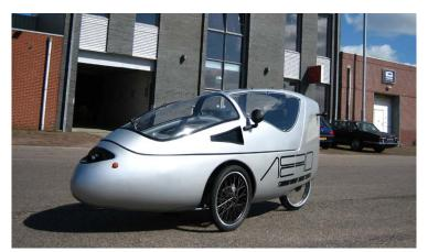
Figure 2.12 Aerorider hybrid electric velomobile (www.vkblog.nl)
