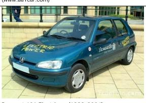
Peugeot 106 Electrique (1998–2004) Maximum speed: 90km/h Range: 80km (www.electroauto.cz)
