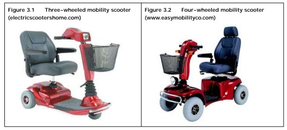
These scooters range in weight from about 50kg to over 150kg. One of the main factors in determining the weight is the size of the batteries, and thus the lightweight scooters have smaller battery packs and less range. Range varies from about 10km to over 40km. Maximum speed varies from about 7km/h to about 19km/h. Some, like the model shown in figure 3.2, are fitted with lights, indicators and stop lights.
