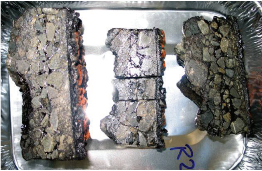
Figure 2.2 Ryan St sample showing how the core was cut. The two halves are the pieces on the left and right, and the centre piece is the ca 20mm slice taken from the right half. Note the small rectangular piece that has been cut in the centre of the slice – this piece was extracted to determine PAH/TPH concentration
