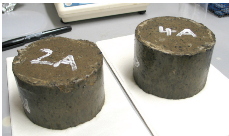
Figure 3.19 Compacted samples of 2A (cement only) and 4A (cement + FB) after 24 h leaching test
