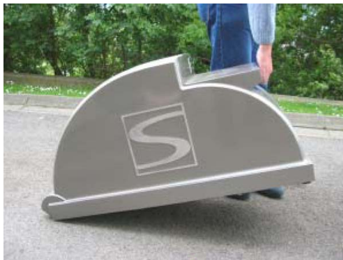
Figure 2.7 'Memphis', the mobile road reflectance gonio-reflectometer
