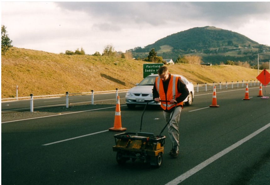
Figure 5.1 GripTester being used in push mode
