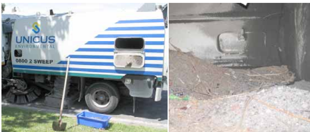
Figure 2.2 Sampling the collected street sweepings from sweeper truck inspection hatch (left) and view of collected sweepings inside sweeper truck (right).
