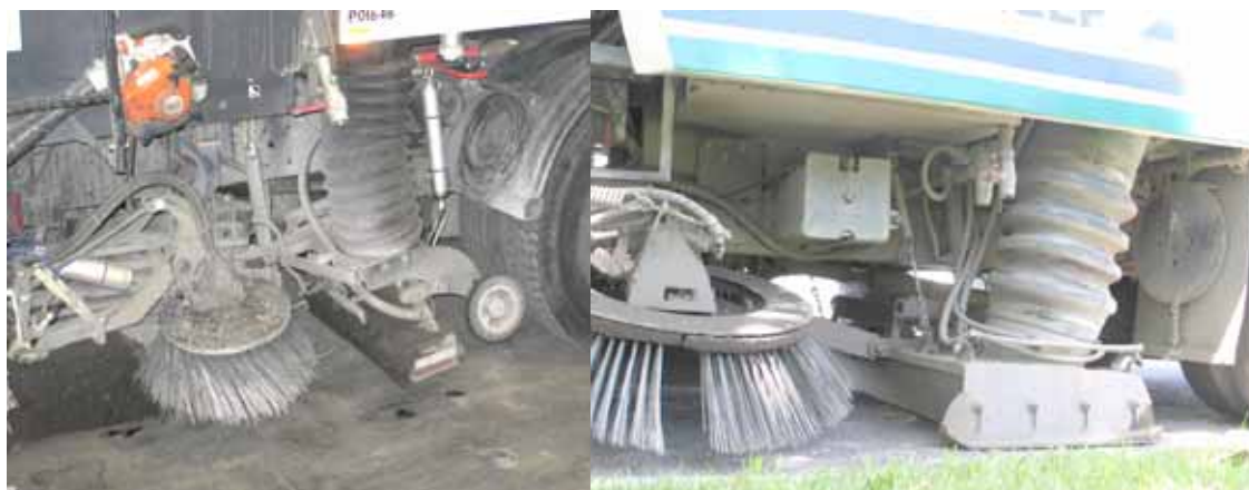
Figure 2.1 The two types of high efficiency sweeping technology used to collect samples – vacuum (left) and regenerative air (right). Note the ‘sweep width’ on the regenerative air sweeper is as wide as the truck.
