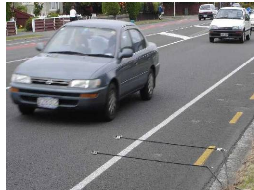
Figure AB.3 Tubes extend 400 mm beyond the cycle lane or edge line.
