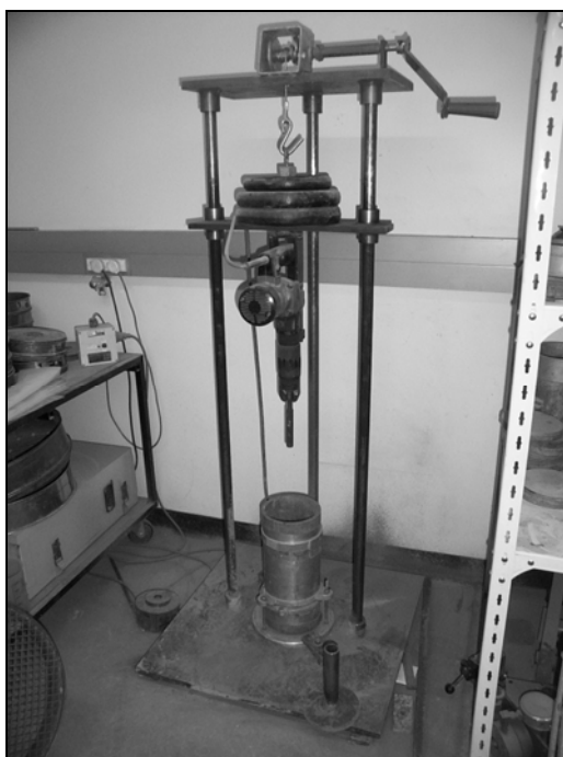
Figure 4.1 Equipment used for compacting RLT test specimens.
