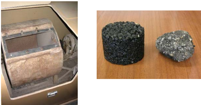
Figure 4.1 Cantabro test equipment and specimens before and after testing.
