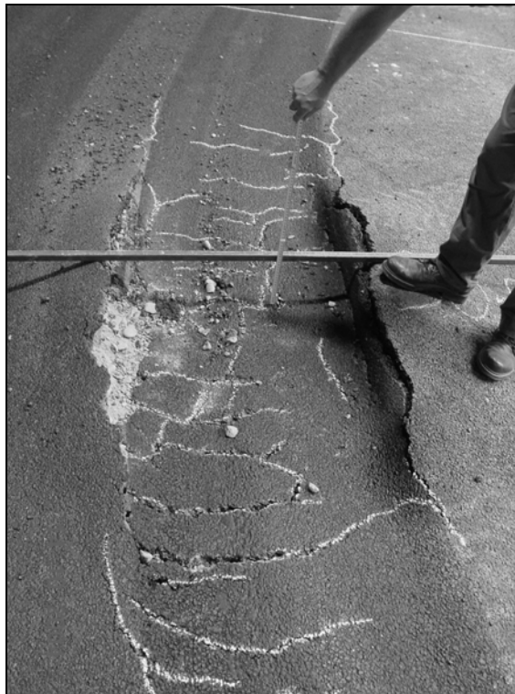
Figure 3.8 Failure at 50 000 repetitions in Section C of the CAPTIF experiment (Alabaster et al. 2006).
