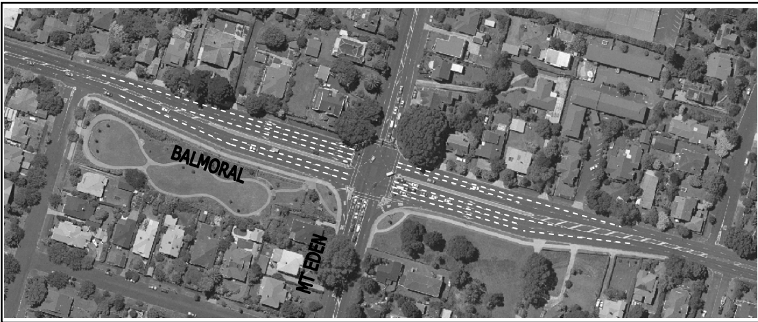
Figure 7.2 Possible road-marking/layout changes for the approach lanes and downstream merges at the Mt Eden/Balmoral intersection.
