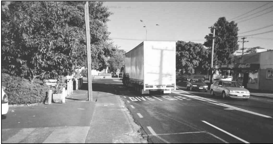
Figure 8.1 Semi-trailer straddling both entry lanes while entering the Frost Road/Carr Road roundabout from the Carr Road approach.
