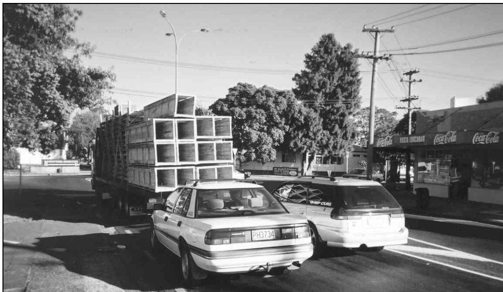
Figure 8.2 Two streams of car traffic following a large truck through the roundabout. Notice that the truck is straddling both lanes.
