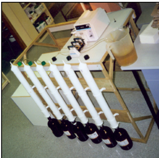
Figure 2.1 Laboratory experiment showing artificial road runoff being applied to six treatment wall columns.
