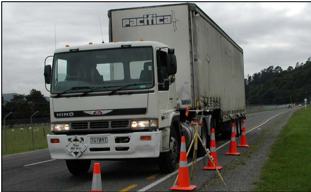
Figure 3.2 The truck used in the experiment was a tractor unit with a 'Taut-Liner' 13 m long semi trailer.
