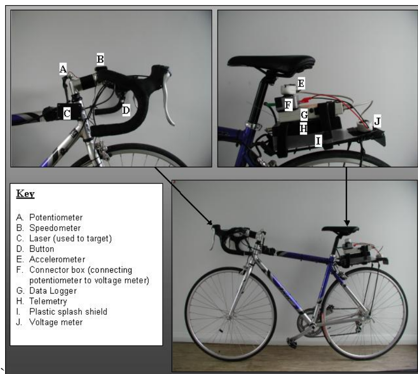
Figure 2.1 The instrumented test cycle used by all participants.
