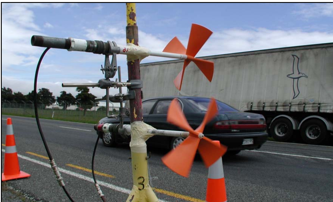
Figure 3.1 Close up of the anemometer arrangement, showing the offset in vertical and horizontal position to minimise wake interference.
