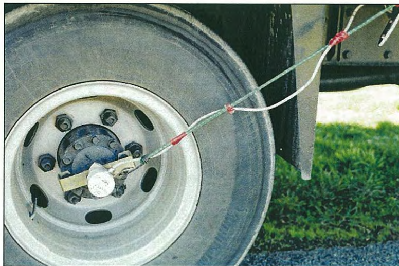
Figure 4.1 Speed profiler device attached to rear wheel of truck.
