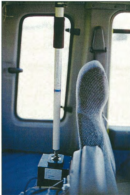
Figure 4.2 Gyro/accelerometer mounted inside test vehicle.
