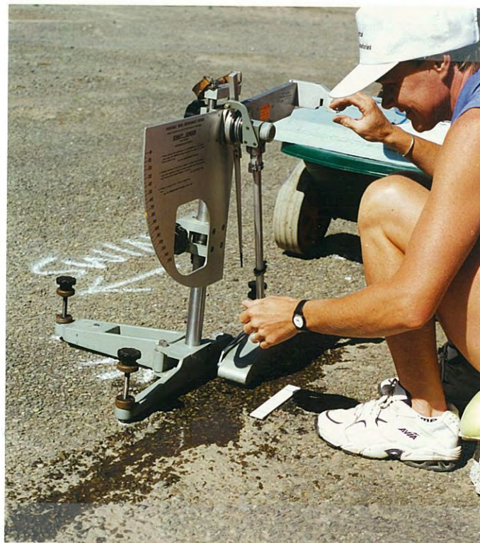
Figure 2. British Pendulum Tester measurement in progress at chipseal site.
