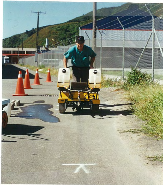
Figure 1. GripTester survey of asphaltic concrete site about to commence.
