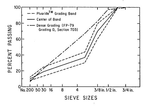
Figure 1. Gradation of PlusRide<sup>TM</sup> aggregate plotted on a 0.45 power graph (reproduced from McQuillen and Hicks 1987).
