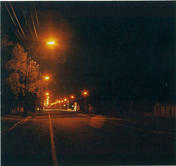
Upper Hutt, Fergusson Drive Camp St to Whakatiki St L=0.23 \text{ cd/m}^2 , U_o=0.34 , TI=34\% Site No. 2
