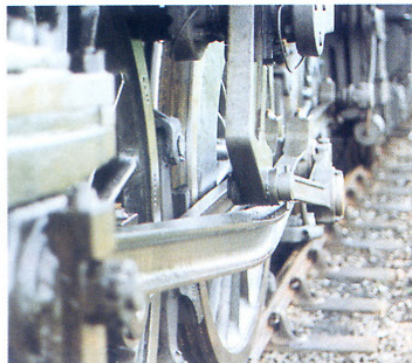
One of the latest incidents, at Fort William on July 13, left BR 'Standard 4' No. 75014 with a badly bent connecting rod and damage estimated to cost £15,000 to repair. This is a classic illustration of the damage that priming can cause.
