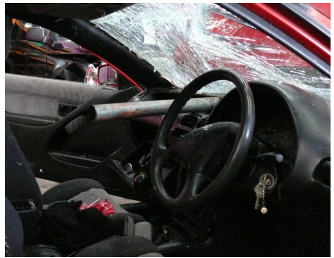
Figure 4: Front passenger area penetration
