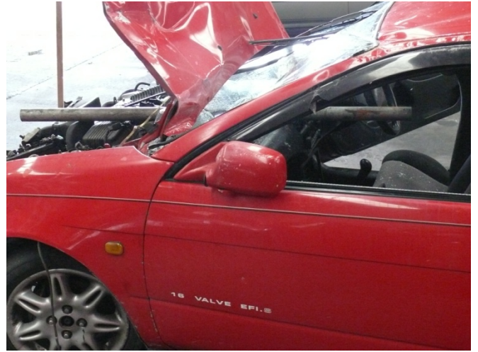
Figure 2: Entry point through front firewall
