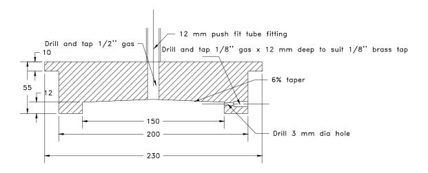
Fig 1: Permeameter Baseplate. Note all dimensions are approximate
