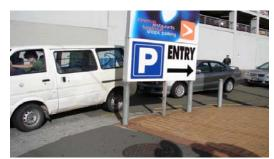
Large car parking sign located at a height that blocks a driver's view of pedestrians stepping out from the footpath
